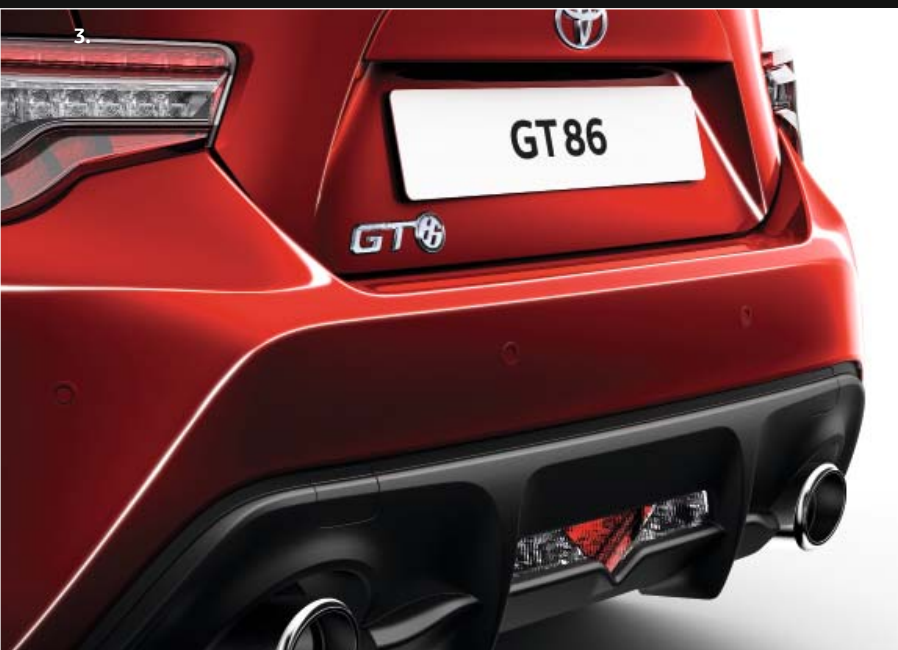
3. Rear Park Assist with ultrasonic sensors and in-car alarm for easier parking.
