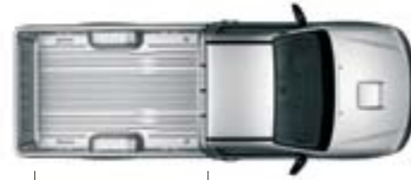
Hilux Single Cab has a deck width of 1520 mm, deck length of 2315 mm and deck height of 450 mm.
