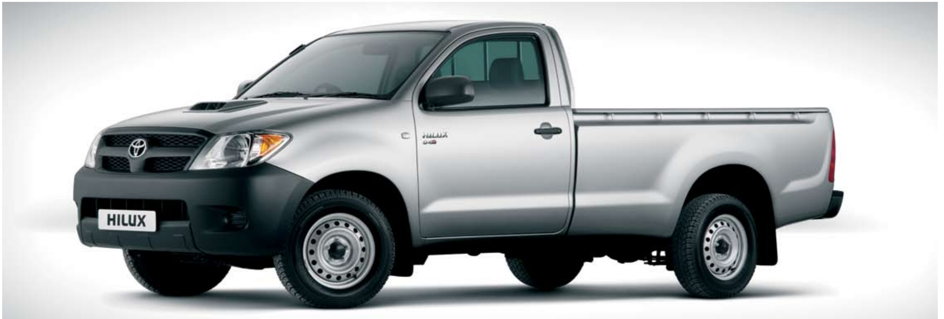
Hilux Single Cab has a deck width of 1520 mm, deck length of 2315 mm and deck height of 450 mm.
