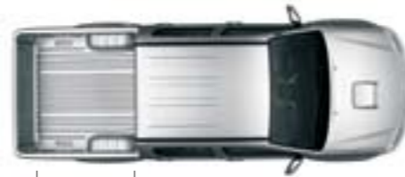
Hilux Double Cab can take a maximum payload of 1060 kg and has a deck length of 1520 mm.
