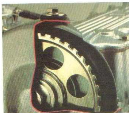
Overhead camshaft is driven by a hard-wearing toothed belt.
