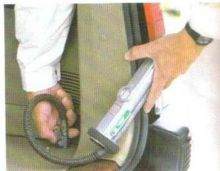
Manual rear suspension levelling is an extra-cost option on Astra L Estate models. This is easily operated by means of a garage air line, and is particularly useful for towing applications or regular heavy payload work. The system ensures that the optimum ride height can always be maintained.
