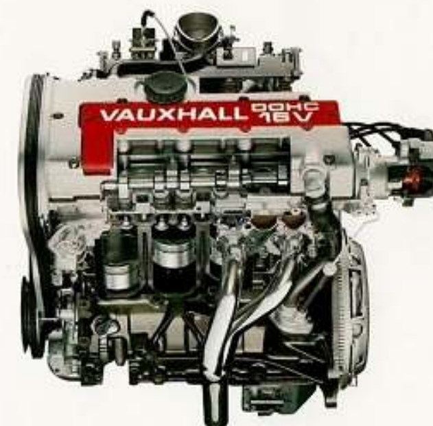
The 150 PS 2.0i 16-valve engine features hollow cam shafts, sodium-cooled exhaust valves and polished cylinder head ports.
