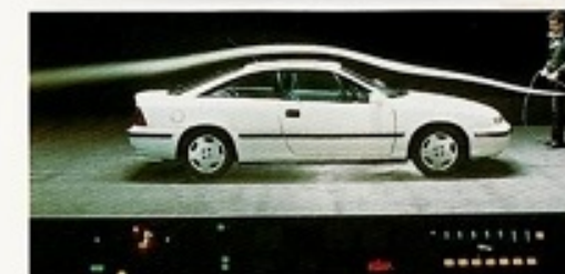
Painstaking attention to detail in the wind tunnel resulted in a 0.26 Cd figure.
