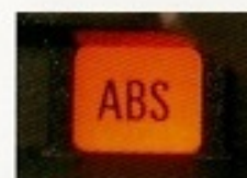
The standard ABS system adjusts braking pressure on each wheel to avoid skidding.
