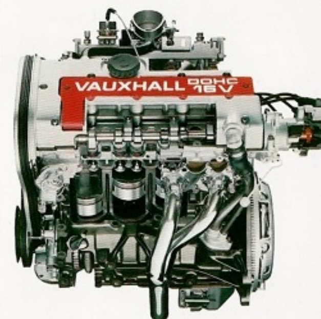
The 150 PS 2.0i Cat. 16-valve engine features hollow camshafts, sodium-cooled exhaust valves and polished cylinder head ports.
