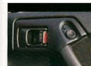
Door mirrors are electrically-operated and heated.
