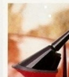
Innovative design - the roof-mounted radio aerial incorporates the rear screen washer nozzle.
