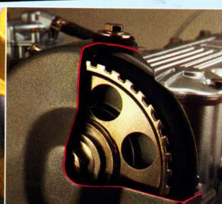
Nova GTE's 100PS 1.6i engine features hydraulic tappets and a toothed cam belt.
