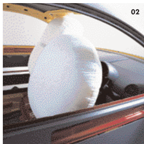
01 The standard side airbags help protect the driver and front seat passenger in the event of a side impact.
