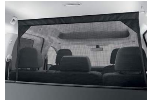
Optional partition net for luggage compartment. An adjustable metal mesh partition grille is also available.
