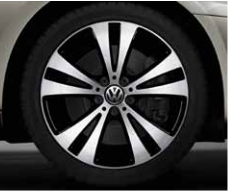
‘Chicago’ 8J x 18 with 235/40 R18 ContiSeal (self-sealing) tyres and anti-theft wheel bolts. Optional on all models.
