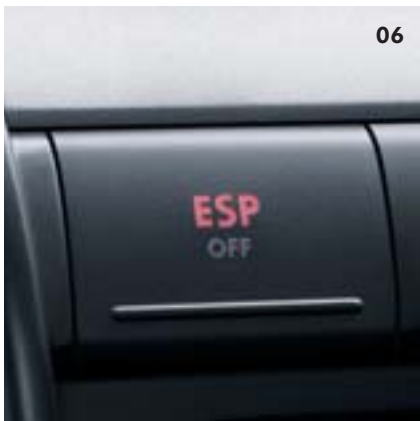
06 The Electronic Stabilisation Programme (ESP) reacts to critical situations within milliseconds and is fitted as standard.
