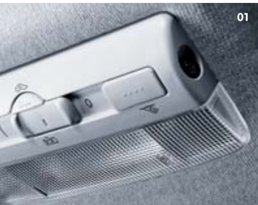
01 The optional alarm with interior protection has a monitor that detects movement in the car and, if appropriate, triggers the alarm.
