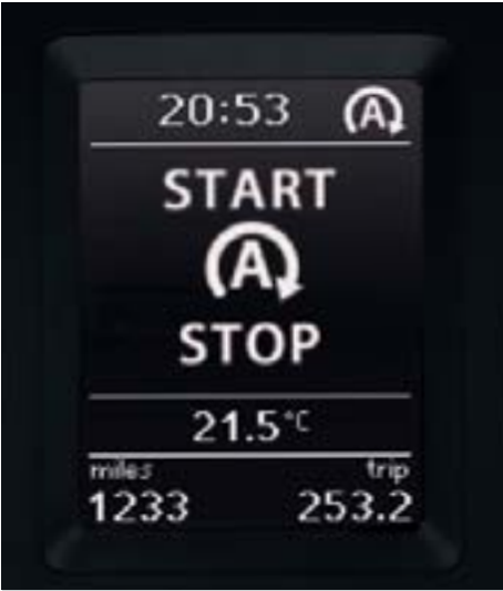
The Start/Stop function momentarily switches off the engine when the vehicle is stationary, in neutral and the clutch disengaged. This is notified to the driver with the ‘Start Stop’ symbol displayed on the multifunction computer (Highline).
