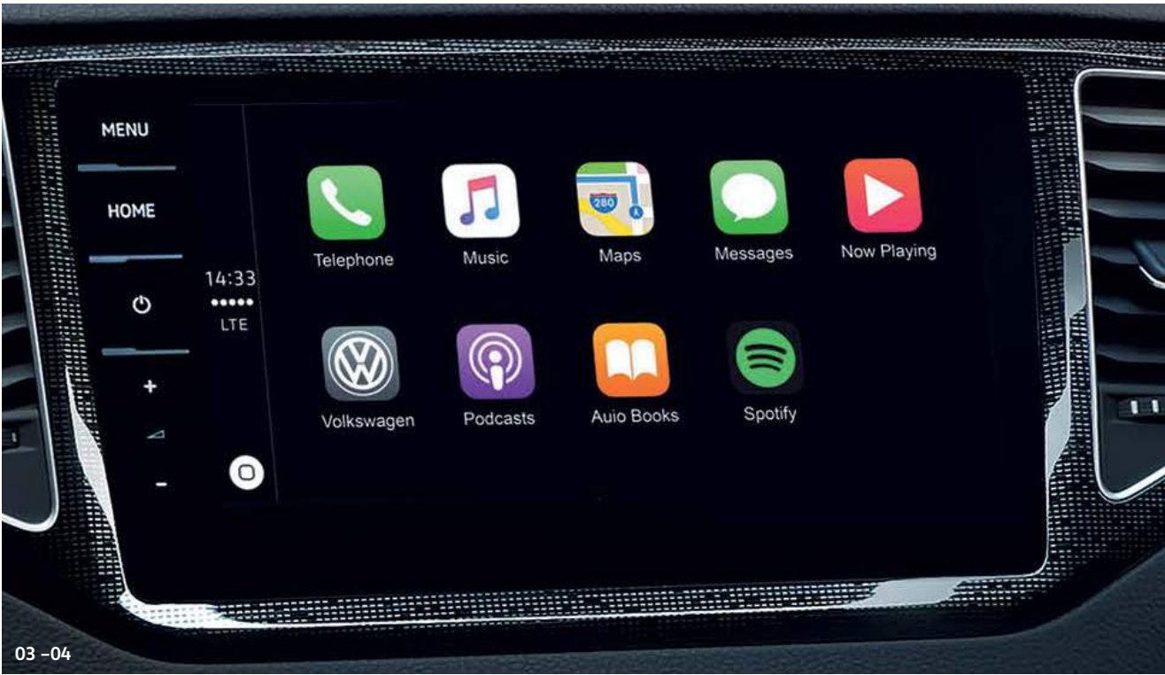
03 The Discover Navigation Pro touch-screen navigation/DVD infotainment system features a glass-covered 9.2 inch colour touch-screen for navigation, DVD, CD and radio functions. It responds to spoken voice commands for navigation and telephone functions, and also features gesture control for use with various different menus, responding to a sideways swiping gesture and confirming a successful swipe with a sound effect, which can be deactivated if required. Building on the Composition Media specification, the system offers Volkswagen Media Control 4 , allowing remote control of the infotainment system via a smartphone or tablet, preloaded European navigation data, 3D map view, three calculated routes (Fast, Short and Eco), dynamic navigation based on TMC+, branded points of interest, Speed Limit Display 2 , photo display from JPEG and PNG files, two SD card readers and a 64 GB SSD hard drive. It comes with 3-years' Car Net 'Guide and Inform Plus' 3 , providing online access to such information as traffic, fuel pricing, weather and news feeds; and includes online navigation software updates, enabling you to download the latest map data. Optional on SE Navigation and GT models.
