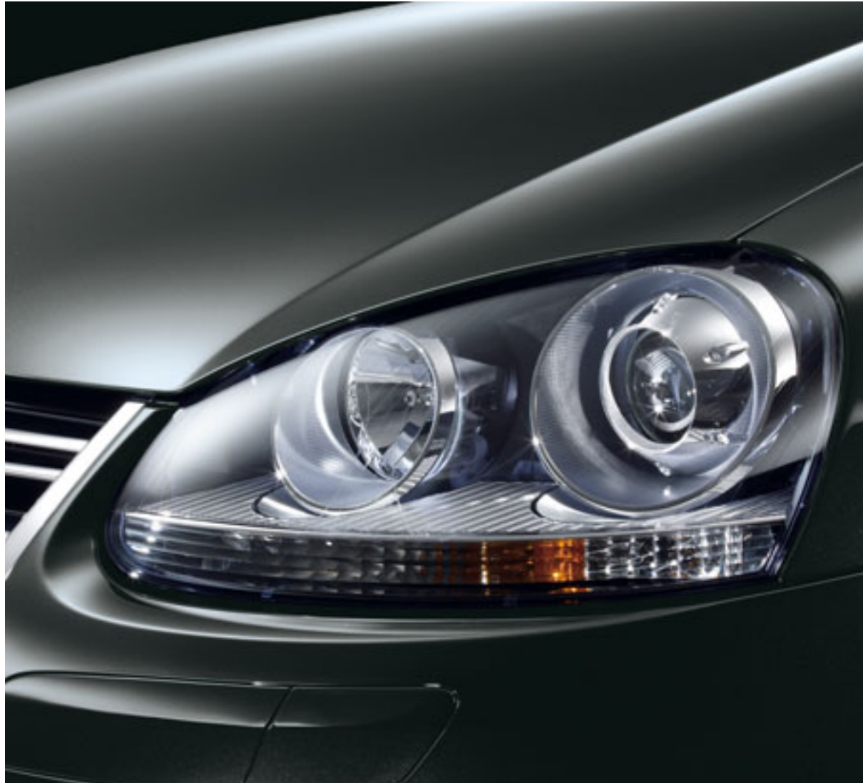
Bi-Xenon headlights including automatic range adjustment and headlight washers produce a brighter, clearer light for both dipped and main beam, giving you a clearer view of the road ahead and helping you to drive more safely. Optional on SE and Sportline models.
