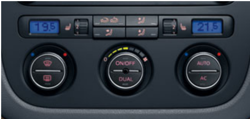
The 2Zone electronic climate control is fully automatic to retain a precise internal temperature and includes automatic air recirculation function. It also benefits from a twin zone setting that allows the driver and front passenger up to 4°C difference in their chosen temperature settings. Heated front seats form part of the Winter pack . Optional on all models.
