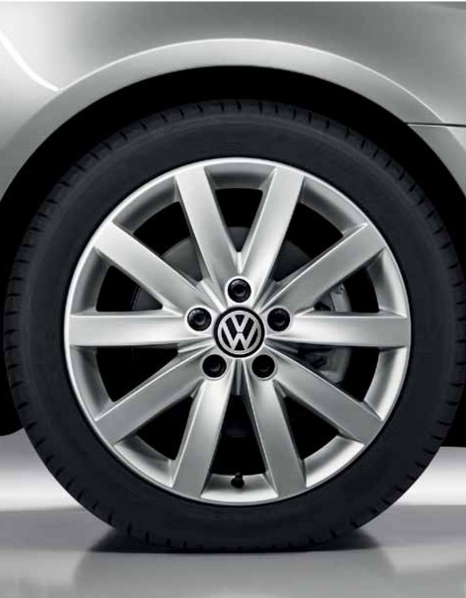
Sporty 17 inch 'Porto' alloy wheels with 225/45 R17 tyres and anti-theft wheel bolts add a great look, while lowered sports suspension ensures safe and assured handling. Standard on Sportline and optional on SE models.
