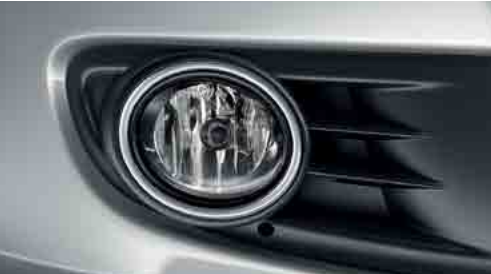
Chrome trimmed front fog lights add a striking look to the front of all Sportline models and include a static cornering function that illuminates the road when indicating or turning at low speed, as well as providing additional safety where there is poor visibility.
