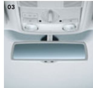
03 Luxury pack – 2 includes the coming/leaving home lighting function. By timer or remote control the headlights and door mirror indicators will illuminate at night-time helping you to find your way in the dark. The pack also includes a rain sensor and an automatically dimming interior rear-view mirror to prevent dazzle from following cars. The exterior door mirrors can be folded back electrically with the driver's door mirror having an automatic dimming function, and the passenger's having a reverse activated kerb-view adjustment. A dusk sensor will automatically switch the headlights on in poor or fading light. Optional on all models.
