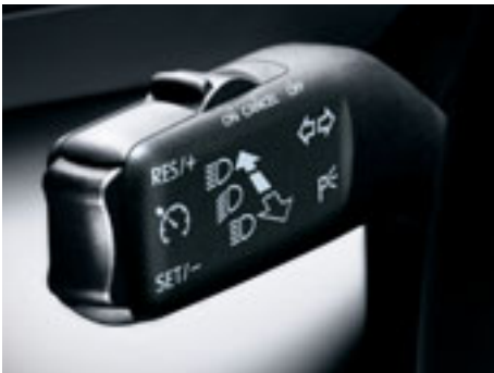
Cruise control, which is standard on SE only, maintains a constant speed, enabling you to relax, particularly on long journeys.
