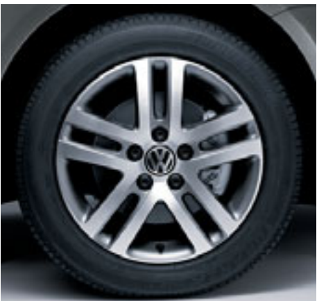
‘Atlanta’ design 6½J x 16 alloy wheels with 205/55 R16 tyres and anti-theft wheel bolts. Standard on SE models and not available as an option.
