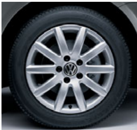
‘Toronto’ design 6½J x 16 alloy wheels with 205/55 R16 tyres and anti-theft wheel bolts. Standard on S models and not available as an option.
