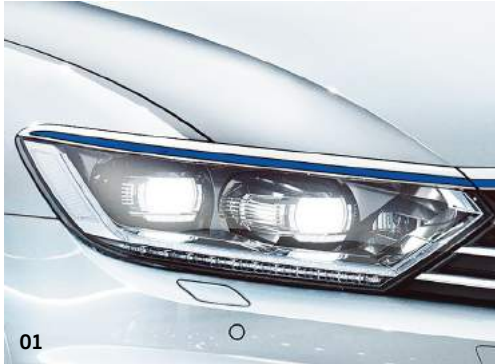
01 LED premium headlights with projection technology include signature dual 'U-shaped' LED daytime running lights and 12 separate LEDs that perform the indicator function. Standard on R-Line models with the 2.0 litre TSI 220 PS or 2.0 litre BiTDI 240 PS 4MOTION engines and optional on R-Line models with all other engines.
