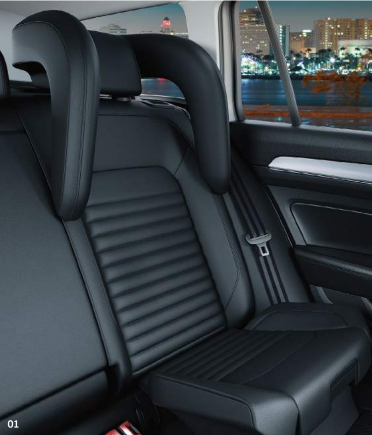
01 Integrated child seats 2 are convenient, practical and easy to use, available for children weighing 15 – 36kg and up to 1.5m tall. Designed to provide optimal side support, they provide a bespoke solution for carrying small occupants. Optional on all models except GTE and GTE Advance. Image shown features optional 'Nappa' leather.
