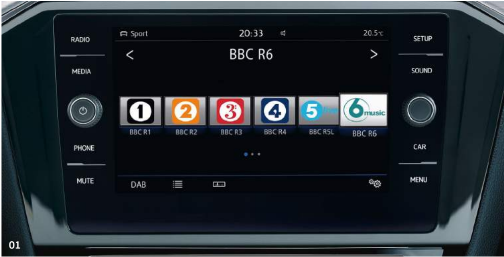
01 The Composition Media infotainment system is equipped with a 8.0 inch colour touch-screen with proximity sensor that recognises in advance your intention to touch the screen and automatically magnifies the display mode. Features also include DAB digital radio receiver, single CD player, MDI (Multi Device Interface) via USB connection for compatible products and SD card reader. The media system also includes Bluetooth telephone and audio connection for compatible devices 1 , simultaneous pairing of two compatible mobile devices, SMS functionality – allowing you to read, compose and send SMS messages using the touch-screen display to a compatible Android smartphone (while the vehicle is stationary), title and compatible cover art display and facilitates music playback from MP3, WMA and AAC files through eight speakers, front and rear. Finally, car information display and ‘Think Blue. Trainer.’ – provide journey analysis and driver tips on your journey. Standard on S and BlueMotion models.
