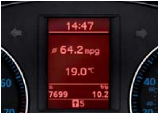
The multifunction computer (Highline) includes visual gear change recommendation for optimum fuel consumption. Standard on BlueMotion Passat Estate models.
