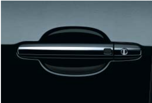
The “ keyless access ” locking and starting system: when the door handle is touched, the electronics of the vehicle communicate with the key. The doors are unlocked and the Memory package activated even if the key is in your pocket.
