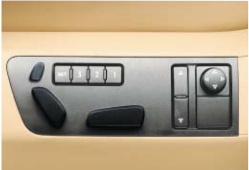
The Memory package for the 12-way seats records individual seat settings, also the positions of the steering column, rear view mirror, door mirrors and seat belts – and adjusts them automatically when the vehicle is unlocked by remote control.
