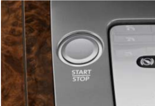
The “ keyless access ” locking and starting system: with the optional “keyless access” function, the Phaeton is started via the starter button without putting the key in the ignition lock.
