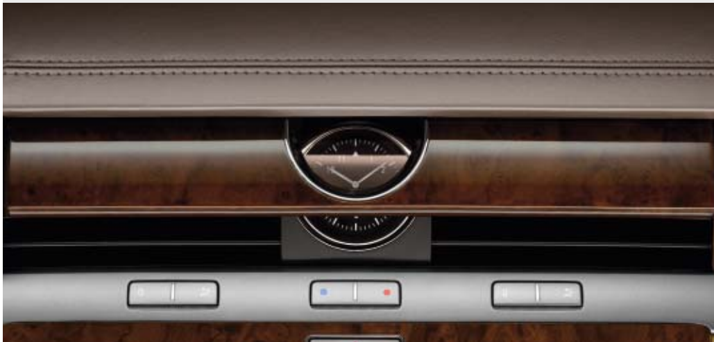
The air vents of the 4-zone Climatronic are opened and closed automatically in automatic mode.
