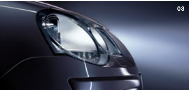
03 The coming home lighting function enables the headlights to illuminate the immediate area after you have exited your car, making it easier and safer when arriving at your destination.
