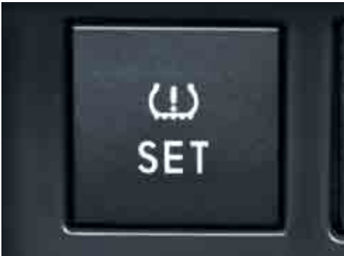
The tyre pressure indicator will alert you to any change in tyre pressure via a warning in the multifunction display, advising you to rectify the situation.
