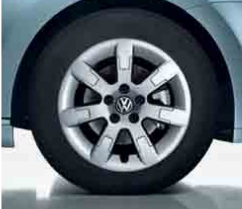
'Greenland' 5½J x 15 light alloy wheels with 185/60 R15 low rolling resistance tyres help to reduce the BlueMotion's fuel consumption. Standard on BlueMotion models.
