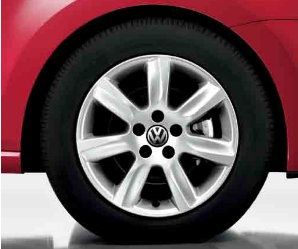
'Greenland' 5½J x 15 light alloy wheels with 185/60 R15 low rolling resistance tyres help to reduce the BlueMotion's fuel consumption. Standard on BlueMotion models.
