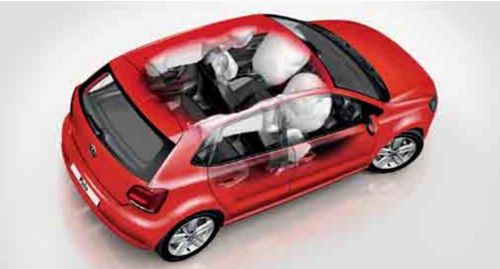
In an emergency situation, all passengers can rely on the safety of the Polo, which includes driver's and front passenger's airbags as well as a side head/thorax airbag system. Deployment of the airbags is activated by crash sensors. When an impact is registered, the airbag control unit ignites the gas generator, which then inflates the airbag within less than 40 milliseconds, helping to reduce injuries significantly. Also available as an option is a curtain airbag system for front and rear seat passengers and front passenger's airbag deactivation, should you require it.
