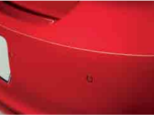
Part of the optional Sensor pack, rear parking sensors emit acoustic signals, alerting you to obstacles in your way when parking: The closer you are to an object, the faster the sound frequency. They also offer a visual display of the vehicle's proximity to obstacles on your radio display.
