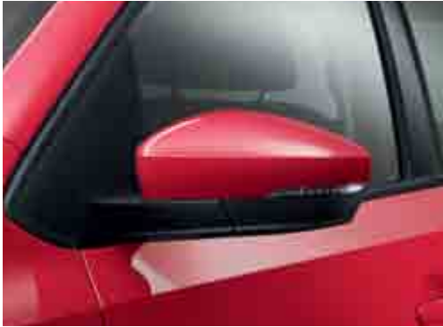
The electrically heated and adjustable body-coloured door mirrors with integrated indicators enhance the streamlined bodyshape and help improve the aerodynamics. Standard on all models except S.
