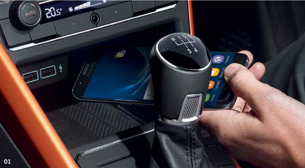
01 The wireless smartphone charger allows compatible smartphone charging without the use of cables. The storage compartment in the front centre console contains a wireless charging pad that you place your phone on top of to charge. The advantage of wireless charging is that it's quicker and easier, as you don't have to plug and unplug each time and, it also looks neater without any trailing cables. Non-Qi-compatible smartphones can be retrofitted with a cover or wireless charging module to allow operation. Please see www.qi-wireless-charging.net for full details. Optional on SE models and above.
