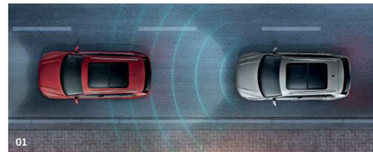
01 Adaptive Cruise Control (ACC) , including Front Assist radar sensor controlled distance monitoring system, City emergency braking system, cruise control and speed limiter offers you intelligent control of your driving speed by automatically adjusting acceleration and braking. Whether around town or on the motorway, the system will adjust your speed to that of the vehicle in front, keep your specified distance, warn if you are approaching too fast and, in an emergency situation, generate enough braking force to try to reduce the severity of a collision or possibly even prevent the collision entirely.
