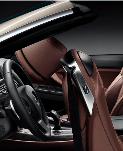
Comfort entry to the rear seats is facilitated by enabling the seatbacks to be released easily with one hand to move the seat back and seat base forward.
