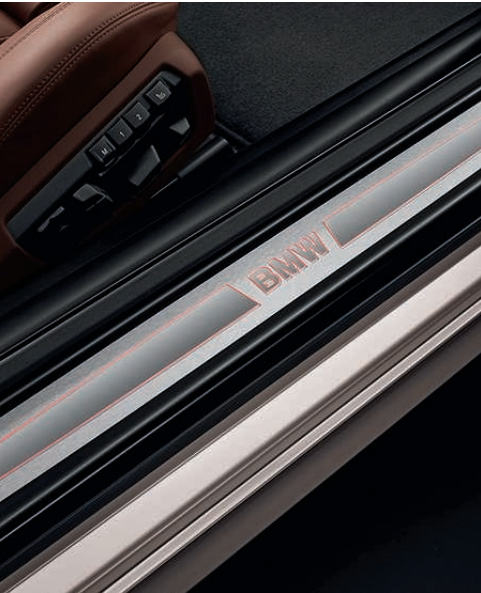
Door entry sills include metal insets finished in high-gloss chrome with a fine-brushed aluminum surround for durability. When the doors are opened, the BMW logo and adjacent strips in each door sill illuminate – a practical and elegant design feature.
