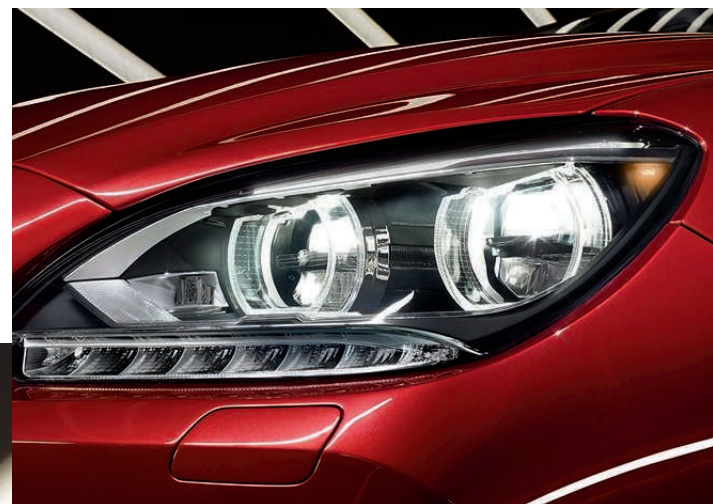
Low and high beams can be generated by available LED technology. As with the Adaptive turning lights and Automatic high beams, the headlights follow the course of the road and adapt to traffic conditions.
