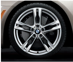
Double Spoke (Style 373M) 20 x 8.5 front, 20 x 9.0 rear light alloy wheels with 245/35 front and 275/30 rear run-flat 1 performance tires 2,3 .
