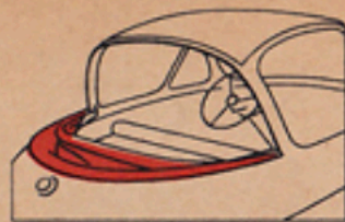
Besides the standard design with canvas hood the BMW Isetta can also be supplied with a convertible hood - in a few seconds the hood can be opened or closed
