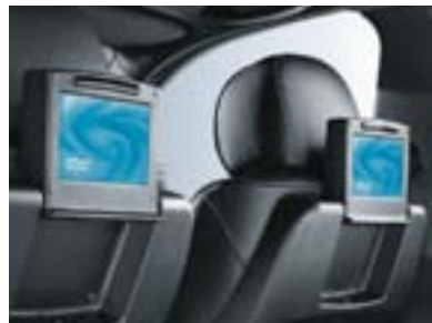
Dual Rear Seat Entertainment System offers two 7" TFT-LCD monitors, Dual DVD players, two wireless headphones and wireless remote.
