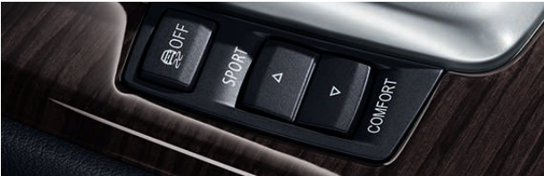
Driving Dynamics Control allows you to tailor the Z4's performance by selecting COMFORT, SPORT or SPORT+ driving modes at the touch of a switch. This changes throttle response, steering assist, suspension damping (with Adaptive M Suspension) and automatic transmission shifting (if so equipped). Additionally, you can deactivate Dynamic Stability Control (DSC) and switch to Dynamic Traction Control (DTC), which allows wheelslip within defined limits when driving in deep snow, or for a sportier driving style. Adaptive M Suspension lowers the chassis by 0.4 inches and electronically adjusts the dampers from sportingly tight to relaxed and comfortable, for greater agility and precise response.
