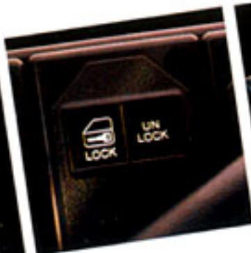
Power door locks.
