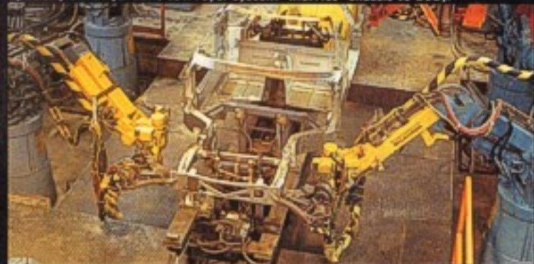
Uniframe components get additional precision robot welds.
