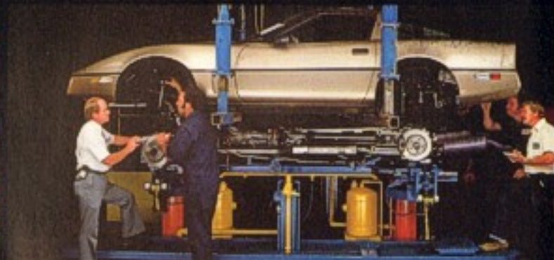
Specially built hydraulic towveer system "marries" chassis to body.
