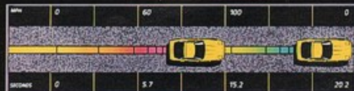
Acceleration and Braking Performance with Manual Transmission
