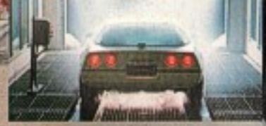
Corvette gets final water test.
