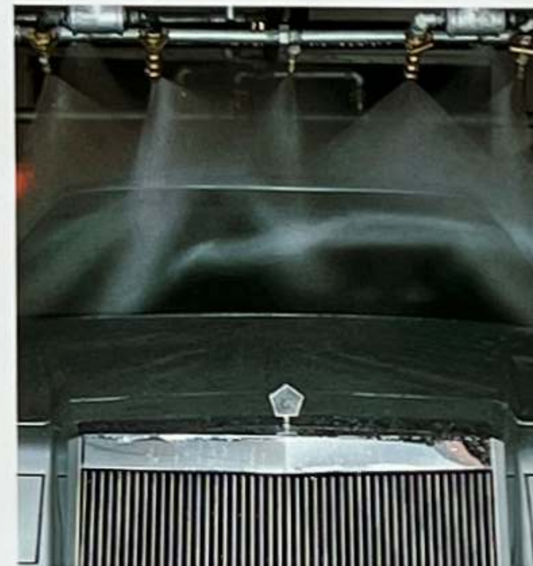
Body panel seals water-tested for leakage.
