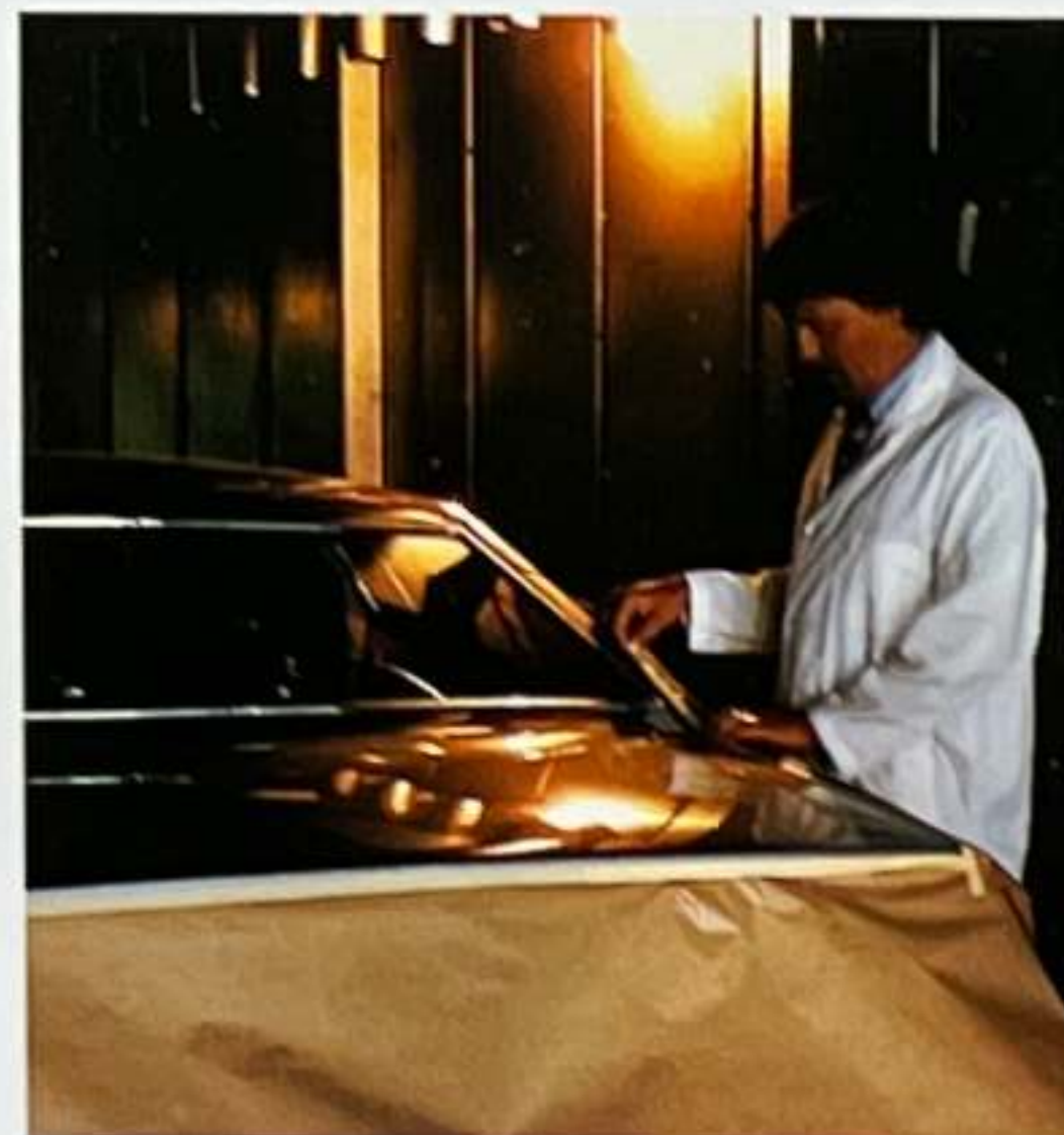
Body paint inspected for flaws.
