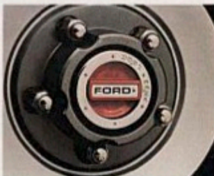
▲ Manual locking hubs are easy to operate. A simple quarter turn of each hub selector to the lock position is all that's needed.
