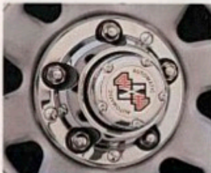
▲ Automatic locking hubs are a standard offering on the F-150.
