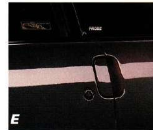
(E) Vertical door handles are flush with the bodysides for smooth air flow.
