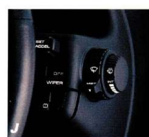
(J) Rotary-type control knobs for windshield wipers and headlamps are positioned for easy operation at the sides of Probe's instrument pod.
