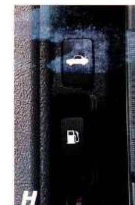
(H) Remote fuel door and rear hatch releases, standard in LX and GT, are conveniently located to the left of the driver's seat.
