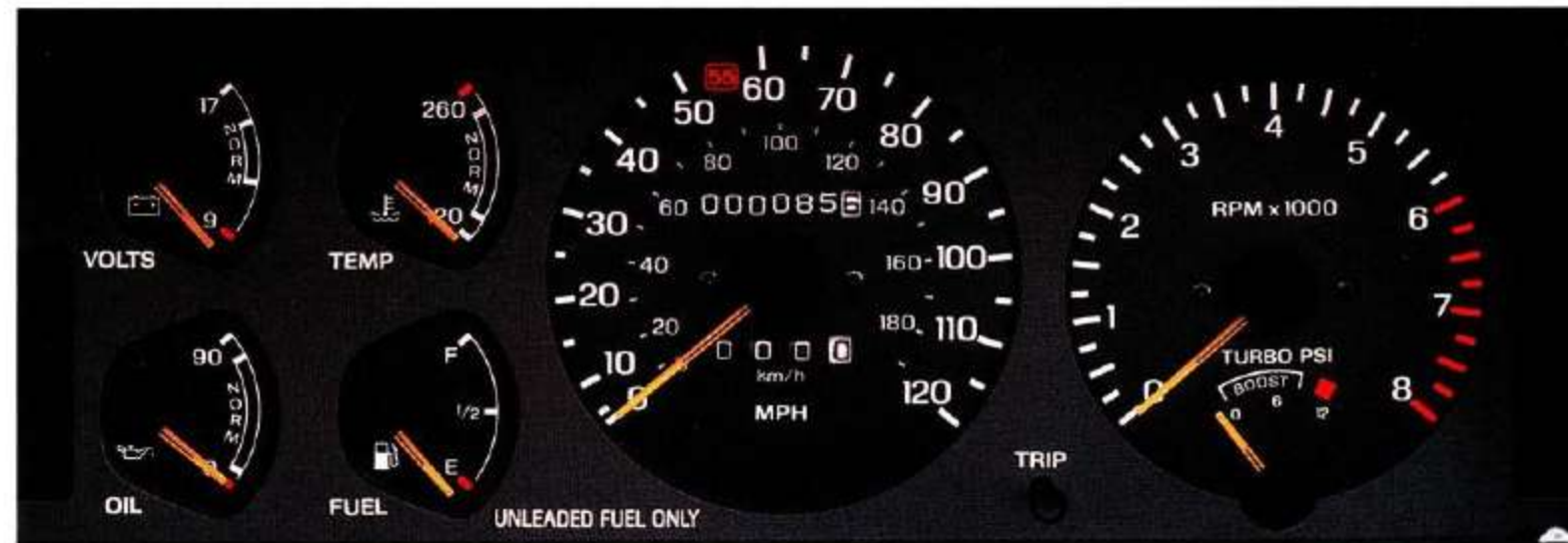
Easy-to-read full analog instrumentation includes tachometer and turbo boost gauge.
