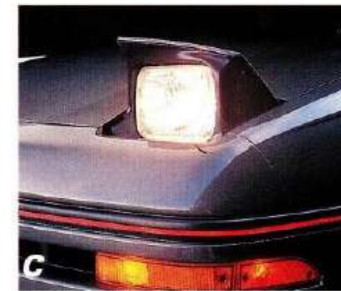
(C) The aerodynamic hood line has concealed/retractable halogen headlamps.
