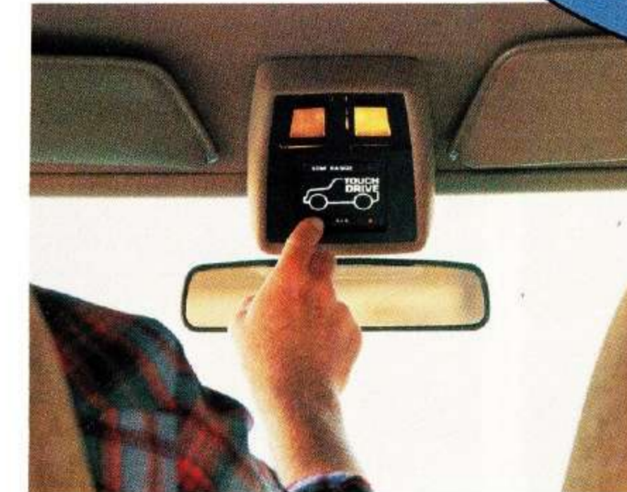
Optional Touch-Drive provides maximum 4-wheel convenience. The automatic hubs engage instantly because an innovative magnetic clutch spins up the front drive system from zero to driving speed in milliseconds.
