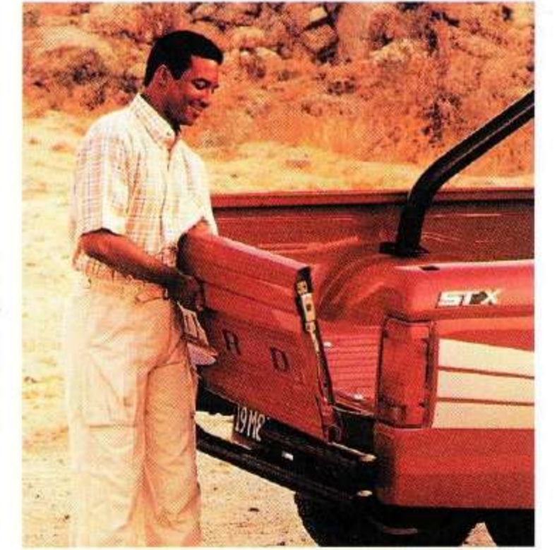
Ranger's tailgate can be removed with ease to accommodate long loads.
