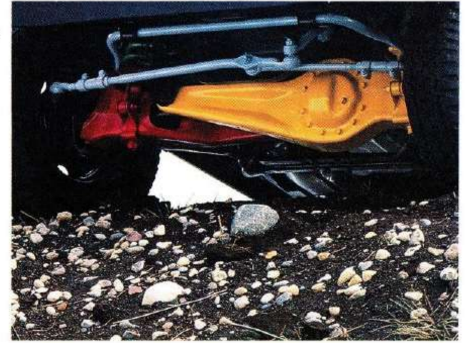
4WD's Twin-Traction Beam front suspension (shown at right and below) allows wheels to step over bumps independently.
