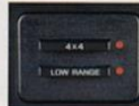
The push-button controls for the standard Touch Drive electric shift transfer case are on the instrument panel — a more convenient arrangement than the floor-mounted shift lever found in other 4x4 pickups. A manual shift transfer case with manual locking front hubs is available in place of Touch Drive.
