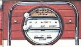
Magic-Aire System combines fresh air heating, scrubbing and defogging into one remarkably efficient unit. The defogger nozzles are specially designed to give even distribution for effective windshield-wide defogging.
