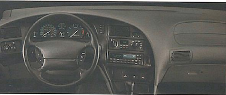
The all-new Thunderbird Super Coupe's instrument panel (above) and steering wheel (right) is DOD. Notice how the dials and controls are angled toward the driver, an important ergonomic design feature. Some adjustment dials, such as the leather seating surfaces, is optional.
