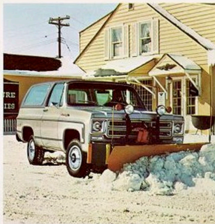
Power take-off with either full-time or conventional four-wheel-drive provides power for utility accessories including rotary brooms and snowplows.
