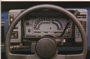
Instrumentation includes a new high-accuracy electric speedometer. Standard full-gage instrument cluster shown. Electronic gage package with tachometer available.
