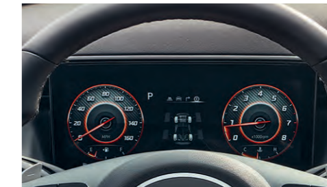
10.25” digital LCD instrument cluster
