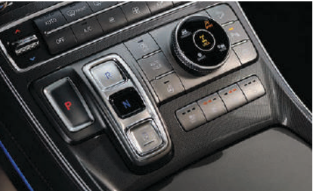
Push-button Shift-by-Wire gear selection
