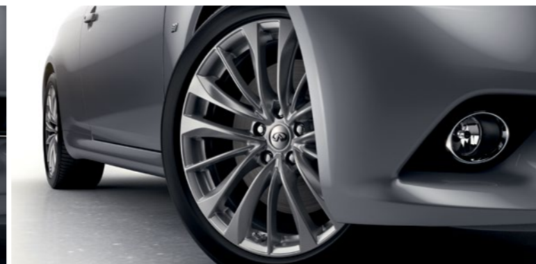
19 X 8.5-INCH (FRONT) 19 X 9.0-INCH (REAR) LIGHTWEIGHT ALUMINUM-ALLOY WHEELS
