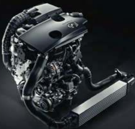
VC-Turbo engine with 268 hp and 286 lb-ft of torque
