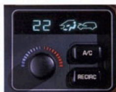
The Automatic Temperature Control system on Grand Cherokee Limited lets you select a degree setting and forget it. Grand Cherokee employs R-134a air conditioning refrigerant, identified as non-hazardous to the ozone layer.
