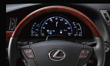
THIN-FILM TRANSISTOR DISPLAY The instrument cluster in the LS 600h L uses an electronic, LED-backlit TFT display to provide the driver with a variety of information, from turn-by-turn directions and hybrid energy consumption to menus where you can personalize select settings for your vehicle.
