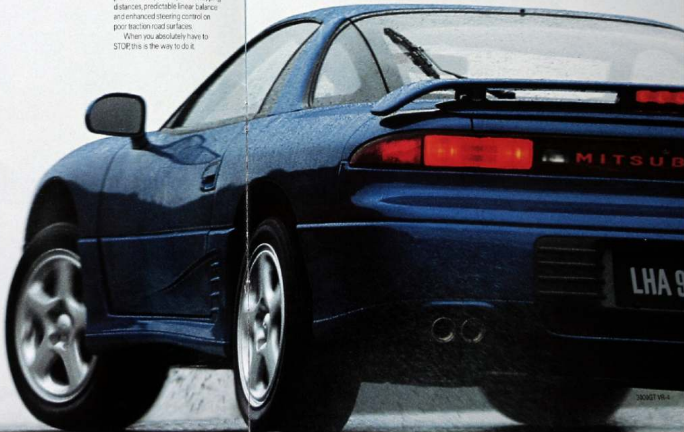
The front air dam and rear spoiler return to their "at rest" position when vehicle speeds drop below 31 mph.
