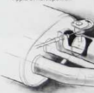
Active exhaust dual-mode muffler.
