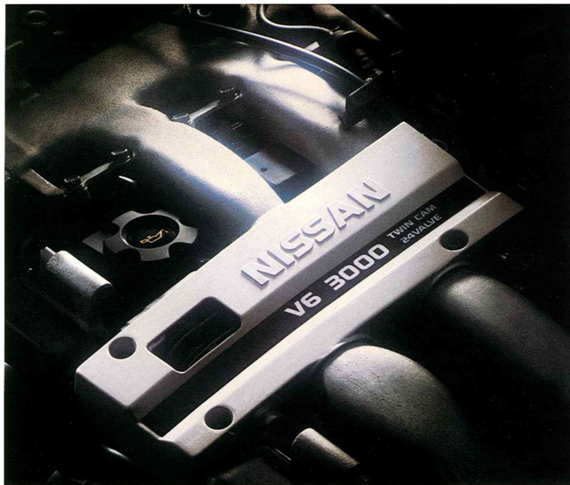
The 222-hp, VG30DE 3.0-liter V6, with its dual-overhead-cam, 4-valve-per-cylinder design.
