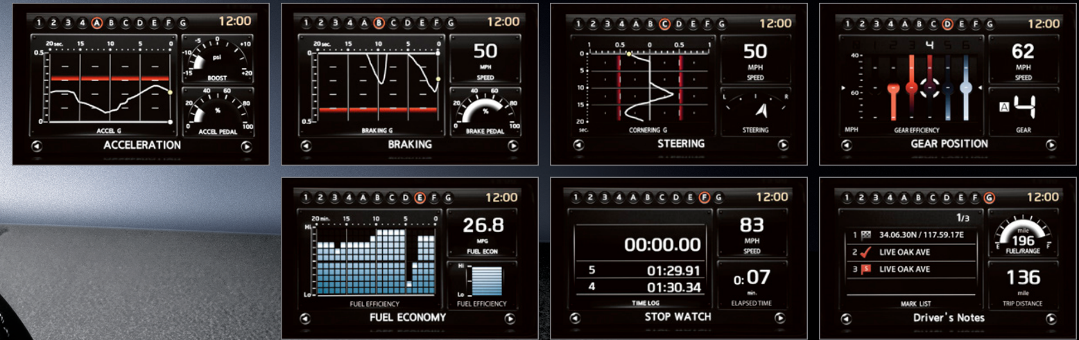
Seven factory preset screens give you quick access to key driving information, including acceleration, braking, steering, gear position and lap time.
