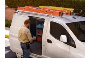
Integrated roof rack-mounting points help secure racks and reduce likelihood of rusting caused by drilling into sheet metal. 1
