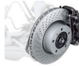
Standard brake system on the 911 Carrera
